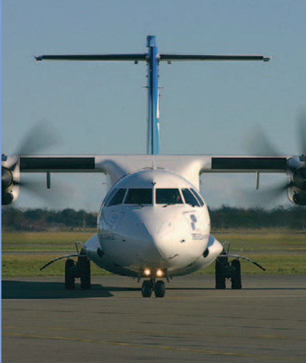
Optimized propeller-fuselage clearance
